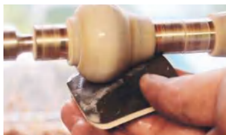
▲ Using the pads wet gives acrylics a high gloss – great for woodturning projects
